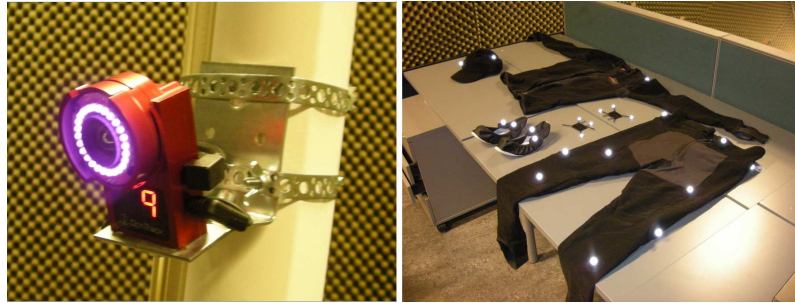
Figure 2.2. On the left is an infrared camera and on the right is a suit with reflective markers that were used for capturing motions.
